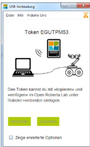
6. Insert the password (token) in the Open Roberta Lab under Robot/Connect and click "OK".
